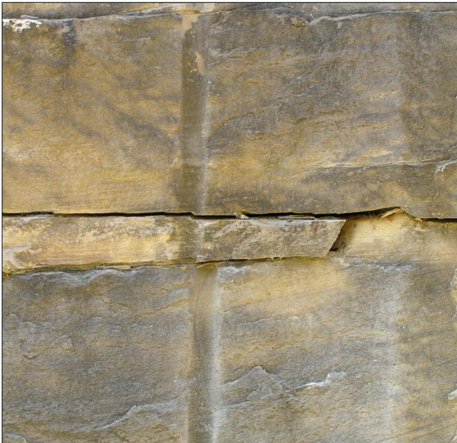
Figure 4: Examples of mining induced shear movements causing offsets and associated vertical fracturing.
