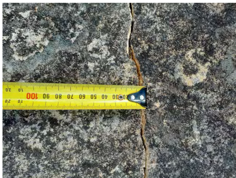
Photo 3: DA3C_LW21_023, maximum width of the rock fracture. Taken: 31/08/2023.
