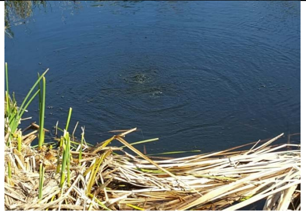
Photo 2: Impact AA7_LW707_001, close-up of gas release observed in property dam. Photo taken 6/04/2016.
