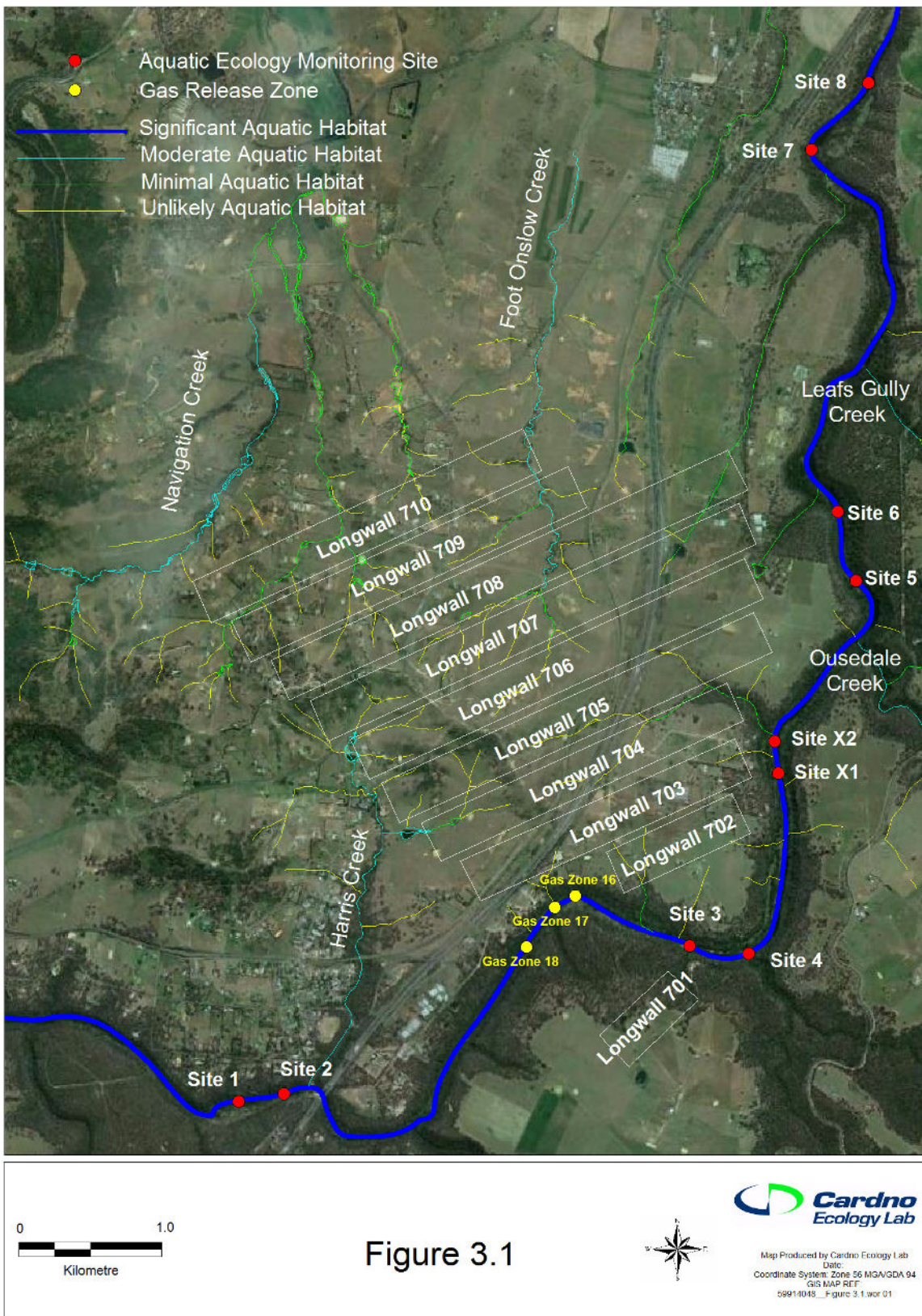
Figure 3-1 Aerial photograph of the study area showing aquatic ecology monitoring Sites 1 to 8 and X1 to X2 on the Nepean River relative to Appin Longwalls 701 to 704 and 705 to 710 and other nearby watercourses. Gas release zones identified during extraction of Longwall 705 are also shown
