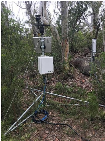
Images 1&2. Initial tripod, logger and STIV camera setup (Left), STIV camera image of CR36S1 (Right)
